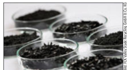
Bild 5: CFK-Recyclate: chopped & milled
